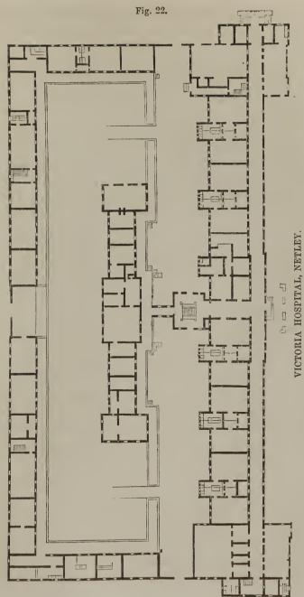
Another objectionable plan, and one which has been extensively used, more or less modified, according to the whim or caprice of the designers, is that in which the wards are arranged on one or both sides of a close corridor. The hospitals at Rotterdam, Hamburg, and Bremen are built after this plan. The wards are small and badly ventilated.
